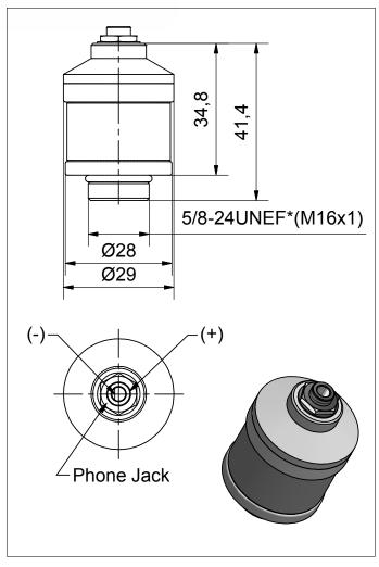
General tolerances ISO 2768-c \*Intermediate thread: Metric / Unified Extra Fine
