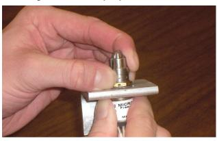
4. Place the lock ring onto the roller guide. The small pin inside the lock ring must be inserted into the hole aligned on the keyway for proper installation.
