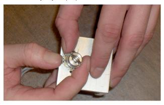
5. Secure the roller guide position by applying pressure with your thumb, directly behind the lock ring pin area, then insert the lock ring into the installed position.
