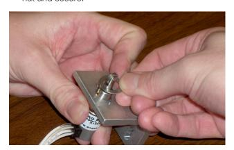
3. Thread the roller guide into the desired position. For easy lock ring placement, align one of the small holes on the roller guide with the keyway.
