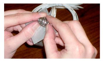
NOTE: The design intent of the lock ring is for a one-time installation. Removed lock rings must be discarded and replaced with new lock rings.
