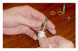
After placing the switch in the intended area, align the internal key washer tab to the bushing keyway and install. Add the internal tooth lock washer, second hex nut and secure.
