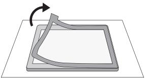
8. Carefully apply the window (tape side down) onto the housing like the previous window.
