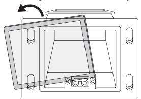
4. Remove remaining adhesive material around the window and clean with isopropyl alcohol and a cotton tipped applicator.
