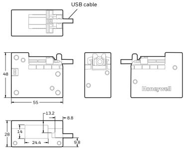
Units are in millimeters. Tolerances: ±0.5 mm.
