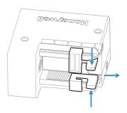
2. Connect a standard USB cable (standard USB-A to micro USB) to the module.
