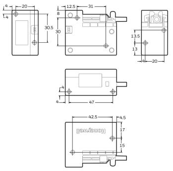
Units are in millimeters. Tolerances ±0.5 mm.
