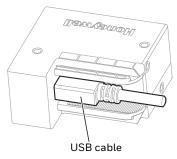
3. Secure the cable to the module using the slider:
