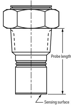
**Figure 13. 3000 Series Housings: Used with Terminations 1, 2a, 2b only**
