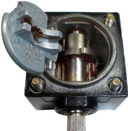
Figure 9. MICRO SWITCH™ LSX Cam Lobe for CCW
