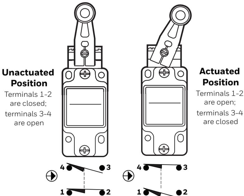
Figure 3. Limit switch normally open/normally closed contacts
