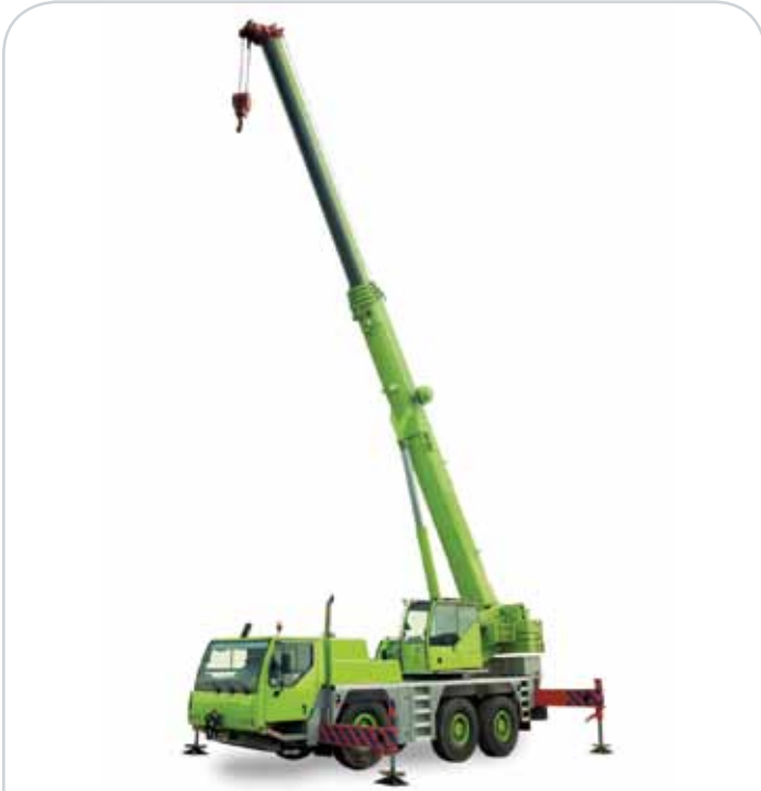
Figure 10. Truck mounted crane outrigger position
