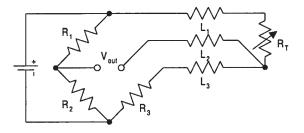
**4-WIRE CIRCUIT:** A 4-wire approach uses a constant current source to cancel lead wire effects even when  $L_1 \neq L_4$ . Use an op-amp to observe V<sub>out</sub> and prevent current flow in L<sub>2</sub> and L<sub>3</sub>.
