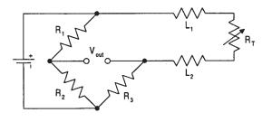
**3-WIRE CIRCUIT:** In this approach,  $L_1$  and  $L_3$  carry the bridge current. When the bridge is in balance, no current flows through  $L_2$  so no  $L_2$  lead resistance is observed. The bridge becomes unbalanced as  $R_T$  changes. Use an op-amp to observe  $V_{out}$  and prevent current flow in  $L_2$ . The effects of  $L_1$  and  $L_3$  cancel when  $L_1 = L_3$  since they are in separate arms of the bridge.
