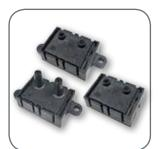
Honeywell Zephyr<sup>™</sup> HAF Series sensors provide a digital interface for reading airflow over specified full-scale flow and compensated temperature ranges. The thermally isolated heater and temperature sensing elements help these sensors provide a fast response to air or gas flow.
