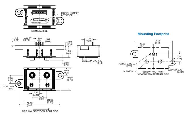
Figure 10. Mounting Dimensions (For reference only: mm [in], continued.)
