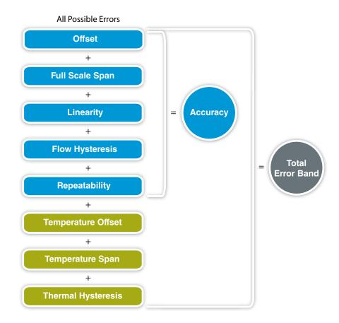
Figure 1. Total Error Band vs. Accuracy
