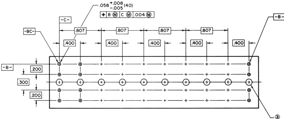
© .125" minimum diameter hole recommended to permit access to annunciator, allowing it to be driven out panel front should replacement become necessary.
