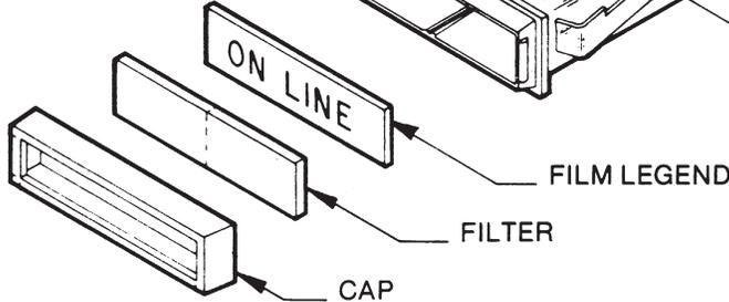
AML45/59 solid state LED annunciators are a state-of-the-art advancement over traditional back-lighted legend displays which utilize incandescent lamps. The LED light source imparts the benefits of solid state long-life and reliability, with low power requirements. Operating life is measured by years, instead of hours.
