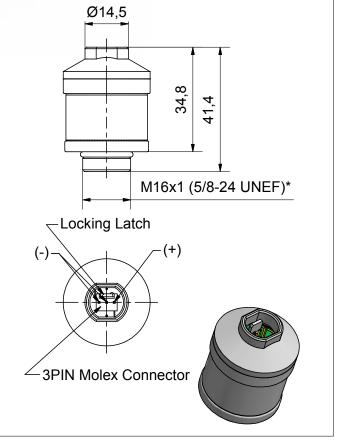
General tolerances ISO 2768-c \*Intermediate thread: Metric / Unified Extra Fine
