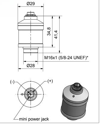
General tolerances ISO 2768-c \*Intermediate thread: Metric / Unified Extra Fine
