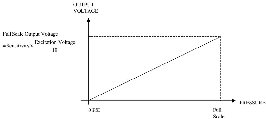
Figure 1 Output Curve
