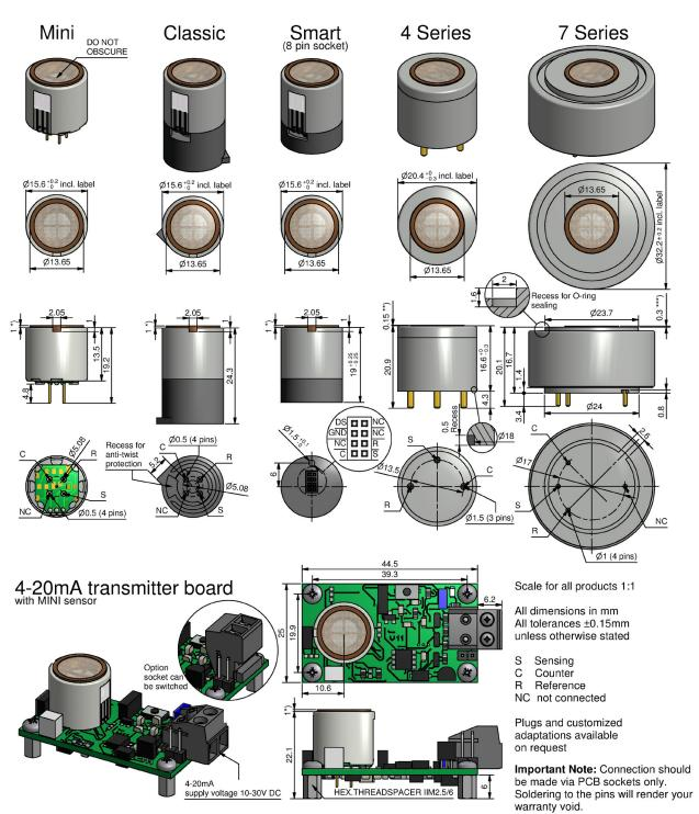
\*) Projection 0.6 - 1.25mm depending on gastype \*\*) Projection up to 0.4mm for 4 Series \*\*\*) Projection up to 0,55mm for 7 Series
