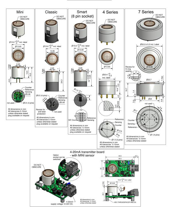
IMPORTANT NOTE: Connection should be made via PCB sockets only. Soldering to pins will render your warranty void.
