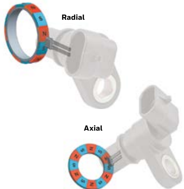
Figure 2. AMR Sensor IC (shown in probe style housing) Mounting Orientation
