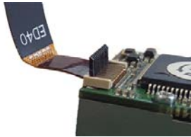
EV14 Ribbon Cable Connector Open
