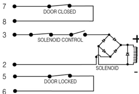
**FIGURE 7. WIRING SCHEMATIC**
