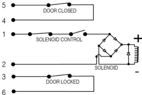
**FIGURE 6. WIRING SCHEMATIC**
