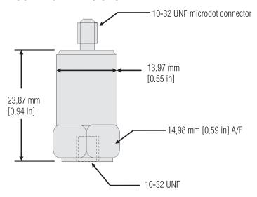
Model MAQ13 Accelerometer
